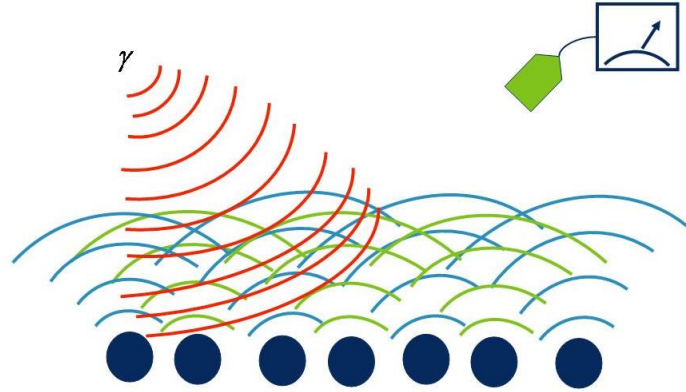
Figure 3.6: Specular reflection as a scattering process: a single photon is simultaneously scattered by all the atoms forming a quantum superposition (the shape and color of the radiated waves are for illustration purposes only, no physical meaning should be given to them).
