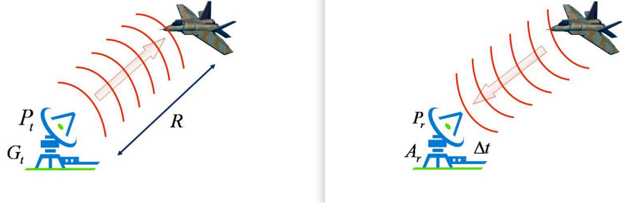
Figure 4.1: Basic operation of a monostatic classical radar. An electromagnetic pulse is sent by the radar transmitter towards the target. The reflected pulse is measured by the radar receiver.
